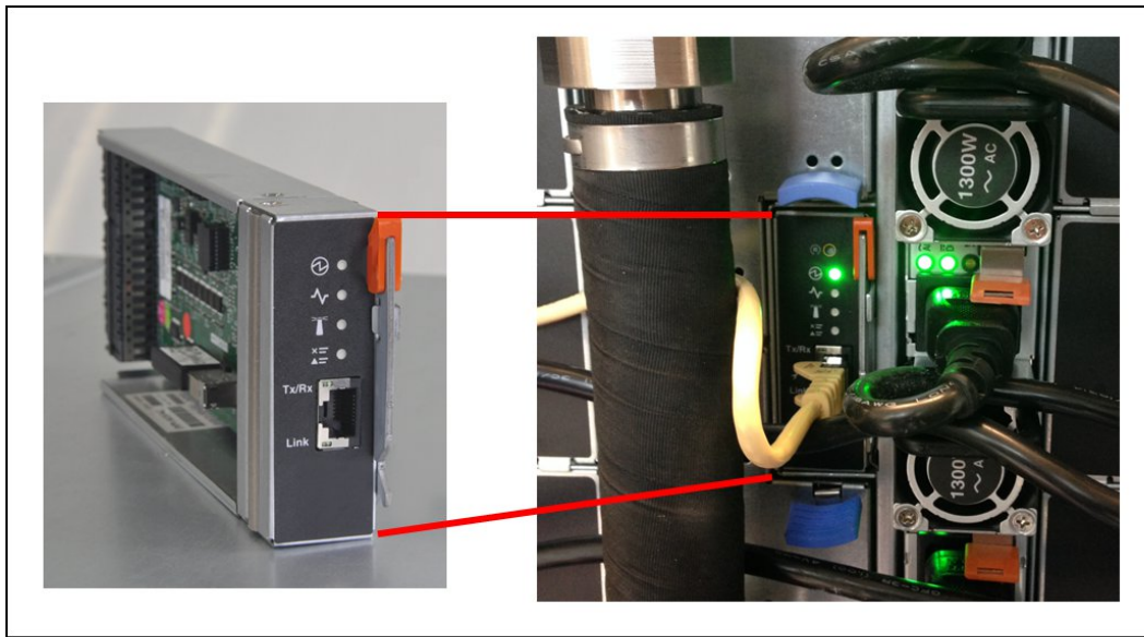
Figure 17. Fan and Power Controller
