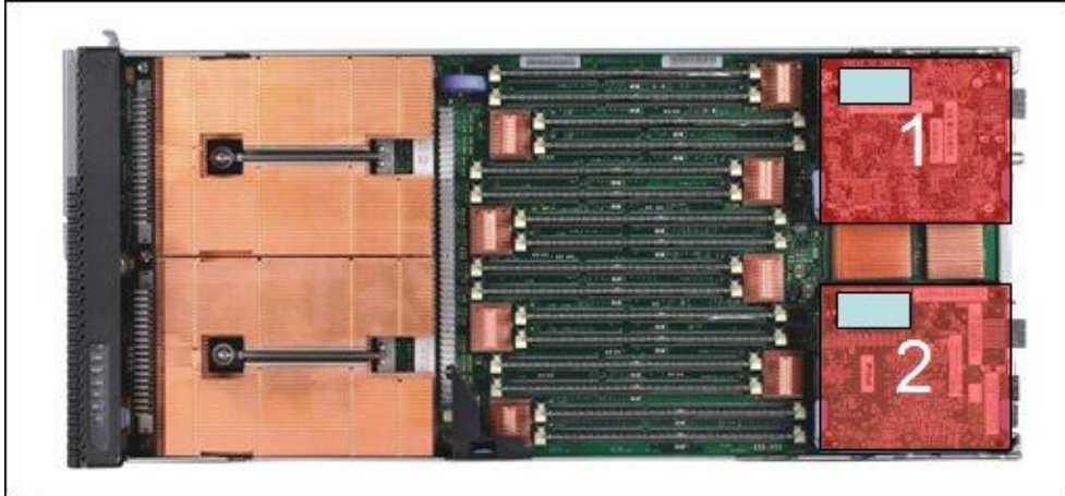
Figure 6. Location of the I/O adapter slots in the IBM Flex System p260 Compute Node
