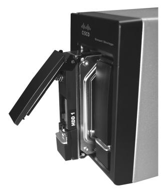
STEP 7 Using your thumb, apply even pressure to the middle of the tray while you insert the tray slowly and fully into position in the chassis.
