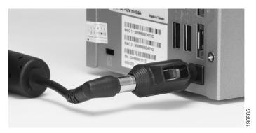
The enclosed DC inline switch module is provided for customers who wish to have a convenient means of turning the device off during extended inactivity. The switch module is provided in compliance with the requirements of the European Union Commission Regulation No 1275/2008. The device is also fully functional without the switch module by plugging the power adapter directly into the device. However, the switch module must be used to comply with the European Union regulations.
