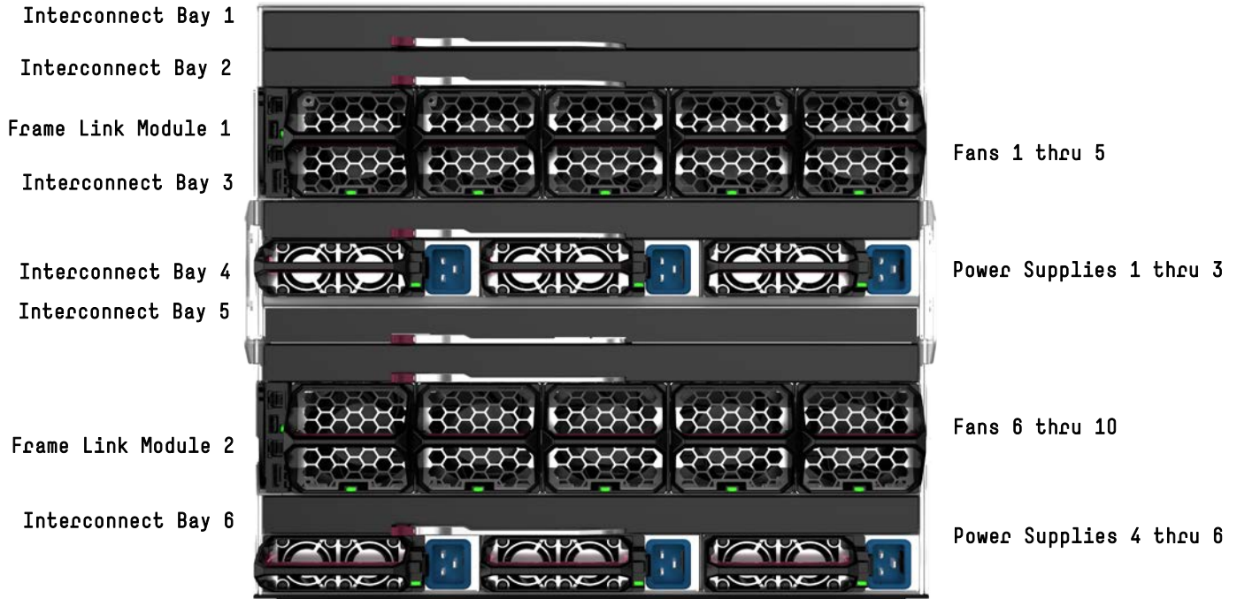
HPE Synergy 12000 Frame - Rear View
