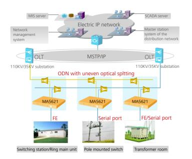
The MA5621 is installed in an outdoor cabinet for remotely collecting and transmitting required information in the electric system. It connects to two optical line terminals (OLTs) by using two PON ports for redundancy protection and connects to the switching station, ring main unit, pole mounted switch, or transformer room by using the FE or serial port.
