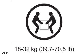
The weight of this part or unit is between 18 and 32 kg (39.7 and 70.5 lb). It takes two persons to safely lift this part or unit. (C009)
