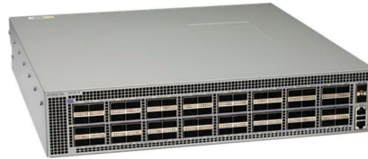
Figure 2: Arista 7260CX3-64: 64x 100GbE QSFP100 ports, 2 SFP+ ports
