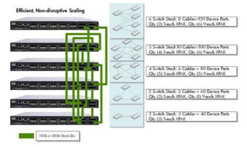
Example of a high availability cable configuration in a single logic FC SAN supporting up to 120 FC device ports
