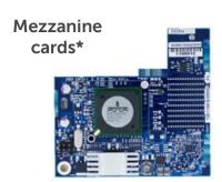
Use Broadcom 5709 dual port server blade I/O Mezzanine Cards in PE blade servers for Gigabit Ethernet I/O connectivity
