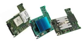
Combine the 10Gb Pass-Through with QLogic QME8142, Emulex OCm10102-f-m, or Intel X520-x/k converged network adapters to the top-of-rack FCoE-enabled switch of your choice
