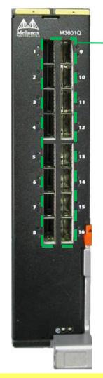
QSFP Active Optical OR QSFP Passive Copper
