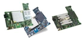
Combine the 10Gb Pass-Through with Broadcom 57710 / 57711 or Intel X520-x/k dual-port 10Gb mezzanine cards for 10Gb Ethernet from server to LAN switch
