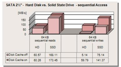
connected to the SATA onboard controller consecutively and measured. The first diagram shows the throughputs for sequential read and write with 64 KB blocks and for different disk cache settings.
