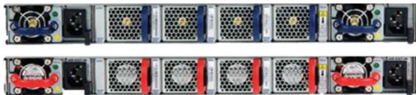
Arista 7050QX 1RU rear view: Front to rear (red) and rear-to-front (blue) airflow
