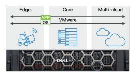
Administrators can choose to deploy PowerStoreOS in a bare metal configuration directly on the PowerStore hardware, or within a virtual machine (VM) running on PowerStore's optional built-in VMware hypervisor, providing yet another layer of isolation, intelligence and abstraction.
