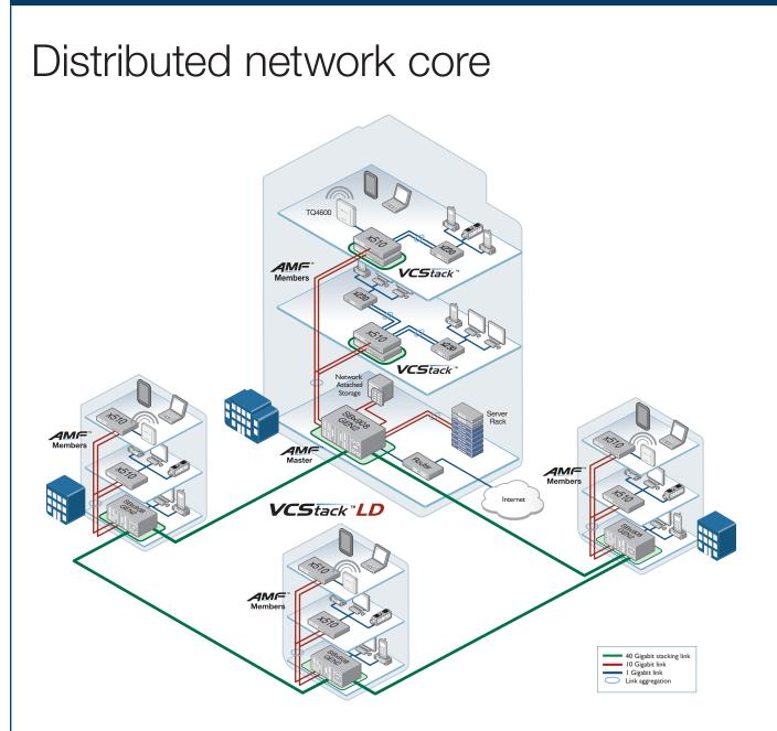
Today's large enterprises demand ready access to online resources and applications, and require a high-performing network that can seamlessly carry multiple converged services. This campus solution uses the SwitchBlade x908 GEN2 and long-distance Virtual Chassis Stacking (VCStack LD)—ideal for a distributed network core that provides high availability, increased capacity and ease of management.
