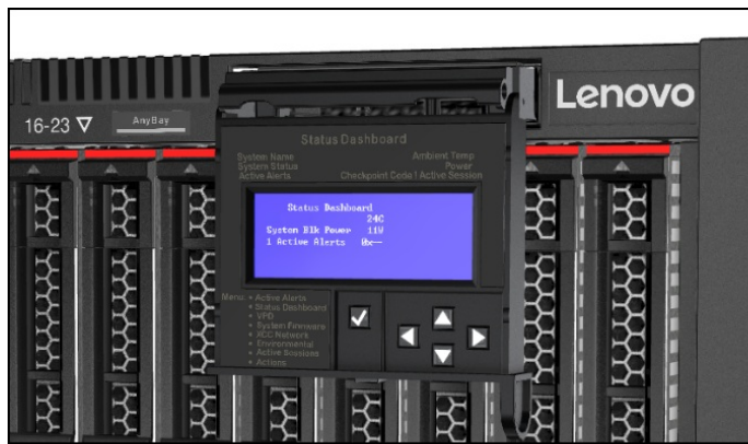
Figure 15. Integrated diagnostics panel with LCD display
