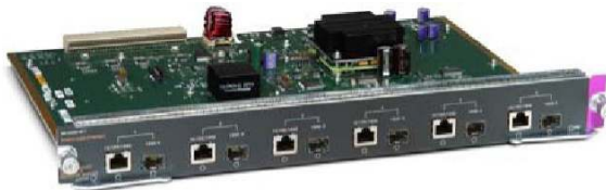
Figure 20. WS-X4506-GB-T Cisco Catalyst 4500 6-Port 10/100/1000 RJ-45 PoE IEEE 802.3af and 1000BASE-X (SFP)
